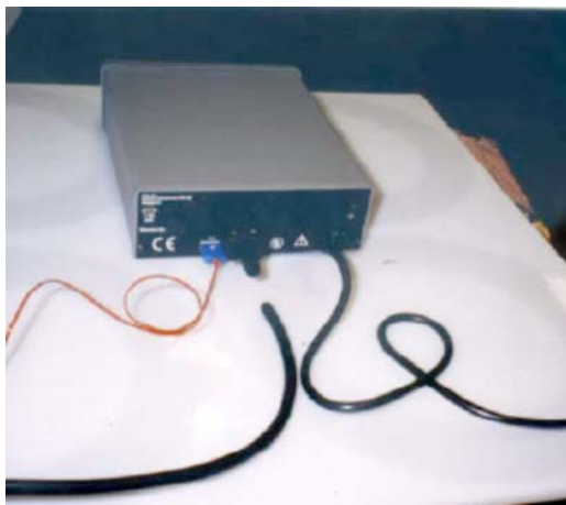
FIG. 9 Controller with connecting Cables: Power Heater Thermocouple
