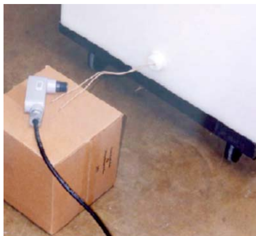
FIG. 7 TC Heater Installed in Tank Exterior
